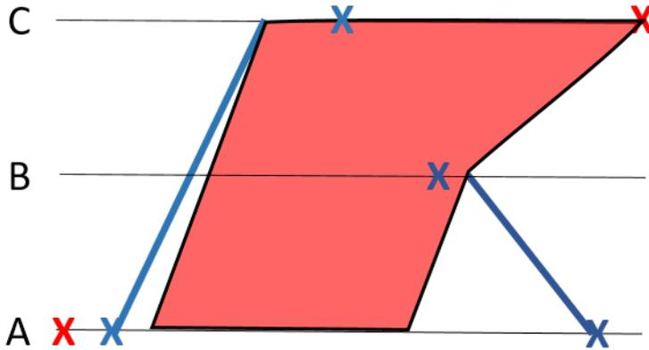
**Figure 7.13:** The number of train paths that fits in on the available track capacity (the red area) is constrained by the most narrow time interval on a station, i.e. the time interval on station A.
