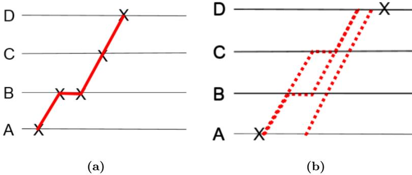
**Figure 2.4:** The difference between a train path and a delivery commitment for a train running from A to D. (a) The operator applies for a train path defined by the crosses. The infrastructure manager has only one option for planning the train path (the red solid line). (b) The operator applies for a delivery commitment defined by the crosses. The infrastructure manager has a number of options for planning the train path. Three suggestions are shown (red dashed line).
