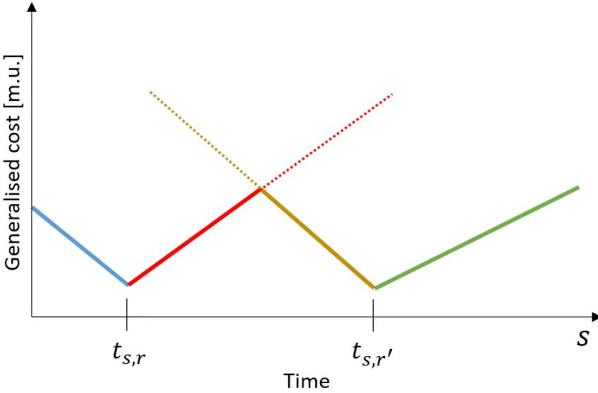
**Figure 6.7:** The blue and red line is the generalized cost for train  $r$  and the yellow and green line is the generalized cost for train  $r'$ . The solid line is the graph of  $\hat{g}(s)$  for the combination of the two trains.
