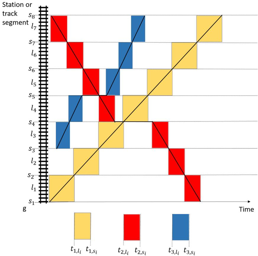
**Figure 4.3:** A train timetable seen as a job-shop scheduling problem. The squares are processes assigned to different machines (or track segments) and the width of the square are the processing times.
