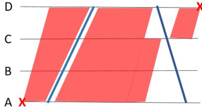
**Figure 7.10:** The available track capacity for a train path application (red area) when the train timetable is constructed of train paths (blue lines). The train paths are fixed in the train timetable and cannot be changed.
