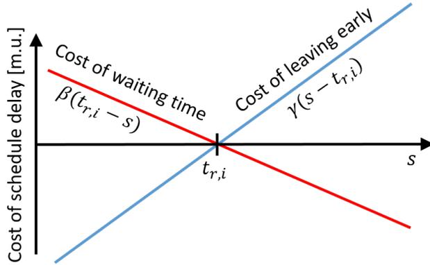
**Figure 6.2:** The cost of schedule delay for a person desiring to travel at time  $s$  and choosing the departure at time  $t_{r,i}$ .
