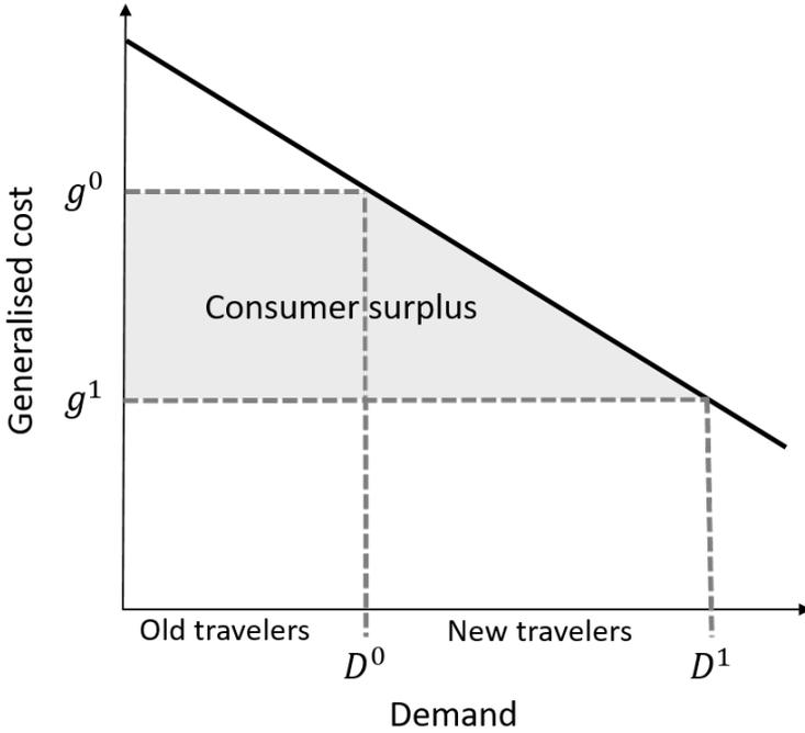
**Figure 5.1:** The relationship between the demand, generalized cost and consumer surplus. The solid line is the demand  $D(g)$  as function of the generalized cost  $g$ . The consumer surplus is the cost "savings" made for all old and new travelers, which is the gray area.
