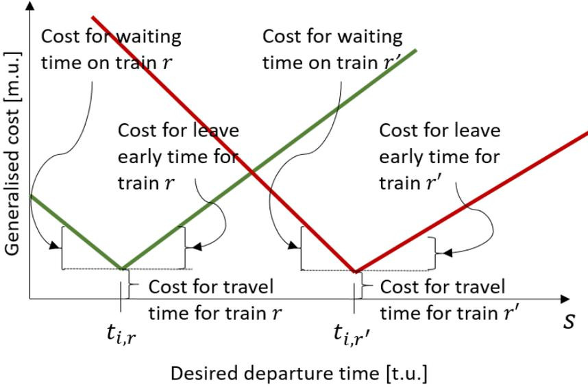
**Figure 6.3:** The generalized cost  $g_{r,i,j}(s)$  for a departure with train  $r$  (green) and train  $r'$  (red) for different desired departure time  $s$ .
