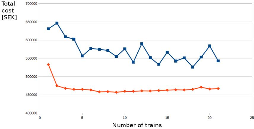
**Figure 6.11:** The total cost before and after the optimization. The blue line is the total cost based on the initial train paths of the train timetable and the red line is the total cost after minimizing the total cost.
