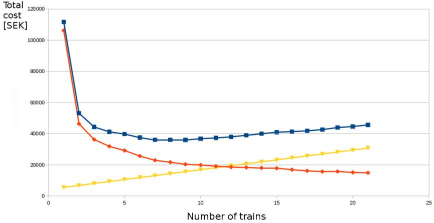
**Figure 6.12:** The costs for different number of train paths on the line. The blue line is the total cost for the line, i.e. the total generalized cost plus the production cost. The red line is the total generalized cost on the line and the yellow line is the production cost on the line.
