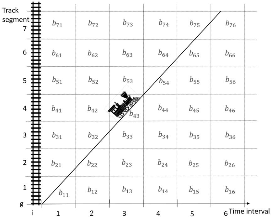
**Figure 4.1:** An example of a time-based model of a railway track. The time and trip are split into track segments and time intervals, respectively. The  $b_{gi}$ -parameters denote the state of track segment  $g$  at time interval  $i$ .
