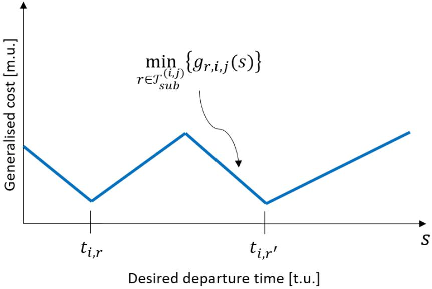
**Figure 6.4:** The generalized cost  $\hat{g}(s)$  for the departure choice of a person desiring to travel at time  $s$ . The cost is illustrated for two trains  $r$  and  $r'$ .
