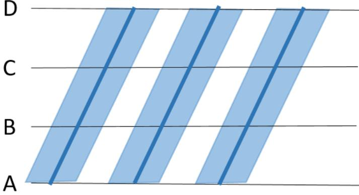
**Figure 6.9:** The blue lines are train paths and the blue parallelograms are the domains. The train paths have to be inside the domains.
