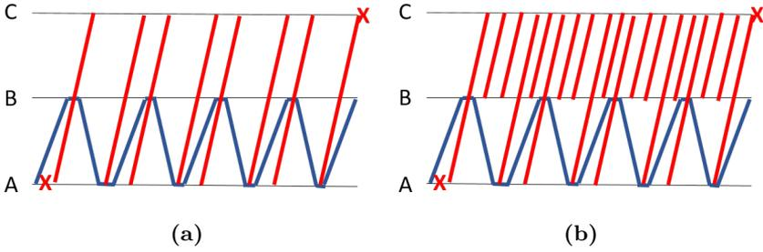
**Figure 7.9:** The delivery commitment application (red) and planned delivery commitment corresponding to a commuter train (blue). (a) The number of train paths is investigated between stations A and C, the traffic between stations A and B and between stations B and C are considered simultaneously. (b) The supply is investigated between stations A and B and between stations B and C separately.
