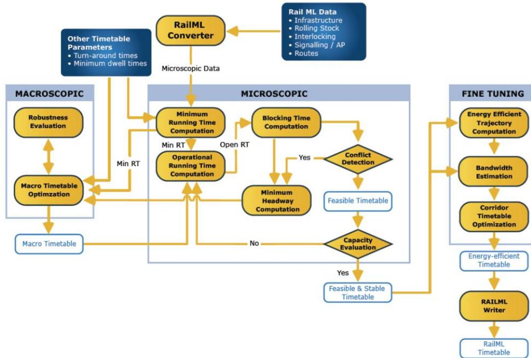
Figure 4. Three level approach to timetabling design provided by the ON-TIME project
