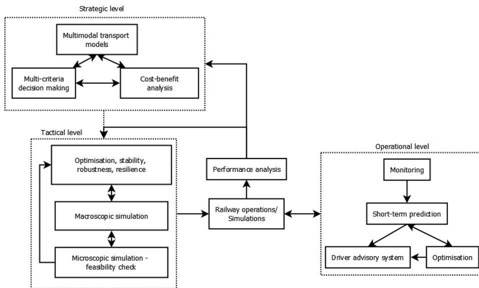
**Figure 6. Existing framework for decision support in planning processes of railway operations provided by the Capacity4Rail project.**
