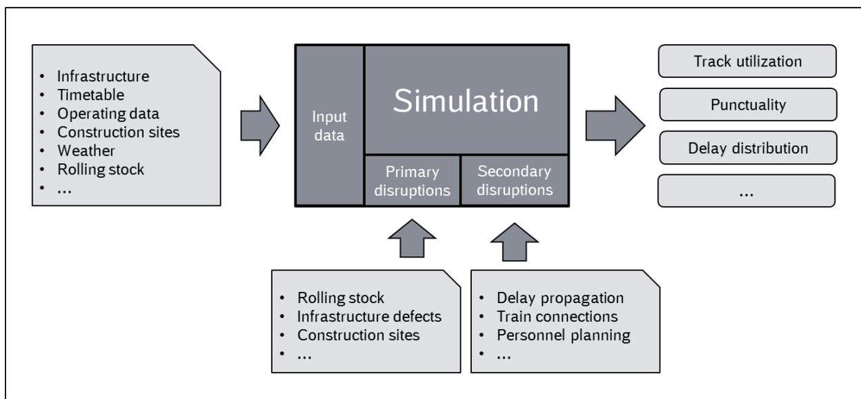
**Figure 12. Draft of the PLASA software prototype.**
