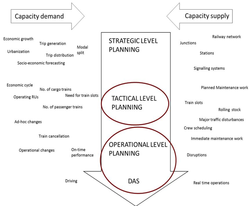
**Figure 5. Aspects of demand and supply of the railway capacity provided by the Capacity4Rail project.**
