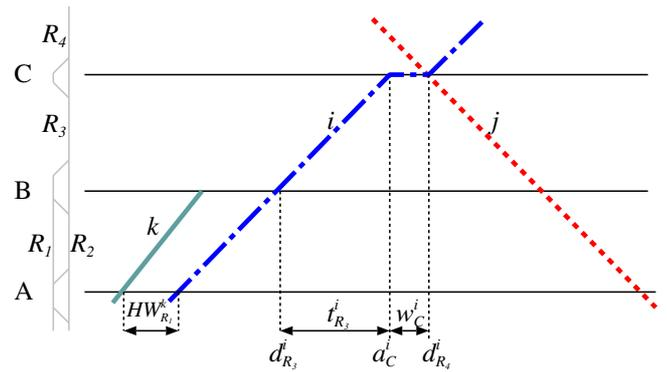
Fig. 1. Three trains  $i$ ,  $j$  and  $k$  scheduled in a network with locations A, B and C and links  $R_1$ ,  $R_2$ ,  $R_3$  and  $R_4$ , with physical layout according to the sketch to the left of the time–distance diagram.
